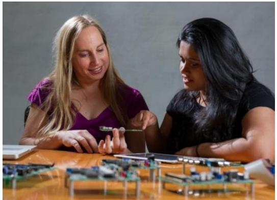
Professor Jennifer Hasler (left) and graduate student Suma George examine a field programmable analog array (FPAA) board that includes an integrated circuit with biological-based neuron structures for power-efficient calculation. Hasler's ...more
