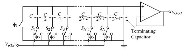
Based on capacitor matching (not monotonic) Charge feedthrough and parasitic issues
