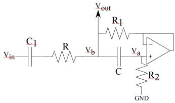
$R = 625\Omega, R_1 = 100\Omega, R_2 = 1M\Omega, C = 1nF, C_1 = 2.5nF$
