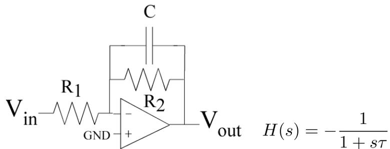
Question 3: (True/False) The circuit has the resulting H(s) transfer function for  $R_1 = R_2$ .
