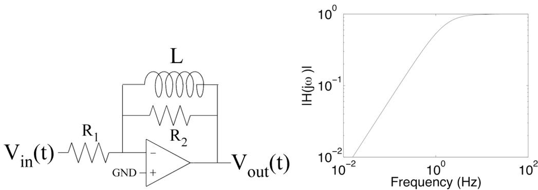
Question 8: (True/False) The circuit has the resulting frequency response shown for  $R_1 = R_2$ .
