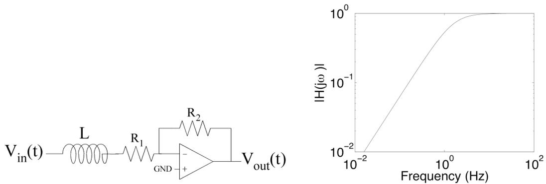
Question 7: (True/False) The circuit has the resulting frequency response shown for  $R_1 = R_2$ .
