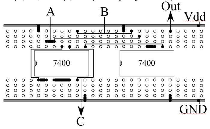
1. Draw the gate level diagram for this circuit.
