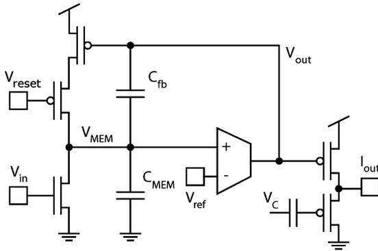
Fig. 9. Integrate-and-fire neuron with synapse output stage.
