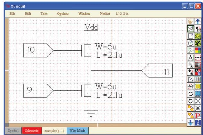
Fig. 7. Xcircuit open source schematic capture tool.
