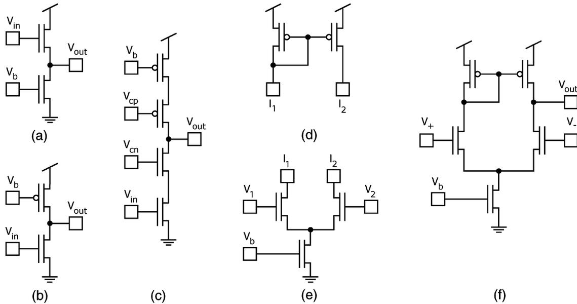
Fig. 8. Progression of circuits synthesized and tested using the FPAA platform. (a) Source follower. (b) High-gain amplifier. (c) Cascoded high-gain amplifier. (d) Current mirror. (e) Differential pair. (f) Operational transconductance amplifier.
