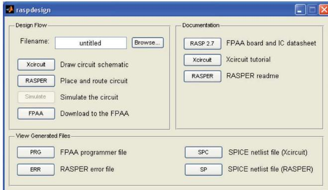
Fig. 6. MATLAB GUI integrating the various tools and software.
