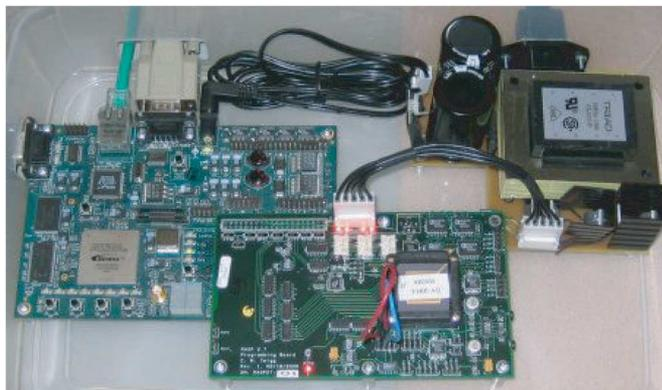
Fig. 2. Self-contained FPAA development platform within a portable box.
