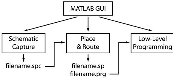
Fig. 5. RASP FPAA design and programming flow diagram.
