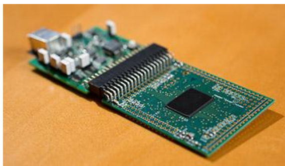
FPAA developed at Georgia Tech by professor Jennifer Hasler as a power-efficient, mixed-signal SoC for neuromorphic computing. (Source: Rob Felt courtesy of Georgia Tech)
