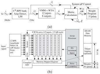
Fig. 9. VMM+WTA classifier Soc FPAA learning algorithm and implementation. (a) Block diagram similar to the tool level description. (b) Structured block diagram illustrating the various required SoC FPAA computations; the target signals and inputs from external and synced together.
