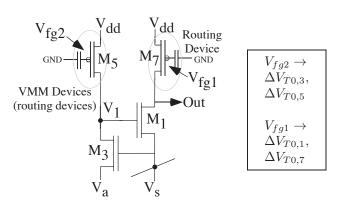
Fig. 5. WTA (+VMM) circuit diagram for addressing mismatch in the classifier structure. The Floating-Gate (FG) voltages can directly account for transistor mismatch for both high-gain sections.
