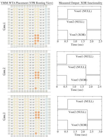
Fig. 6. The XOR classifier data is repeated for the VMM at three different locations, as seen by the three VPR routing views, and similar results. Multiple locations show the calibration eliminates effects of  $\Delta V_{T0}$  due to indirect programming. The location of the VMM weight matrix has little effect on the resulting computation due to initial measurements that calibrate the V<sub>T0</sub> mismatch from indirect programming.
