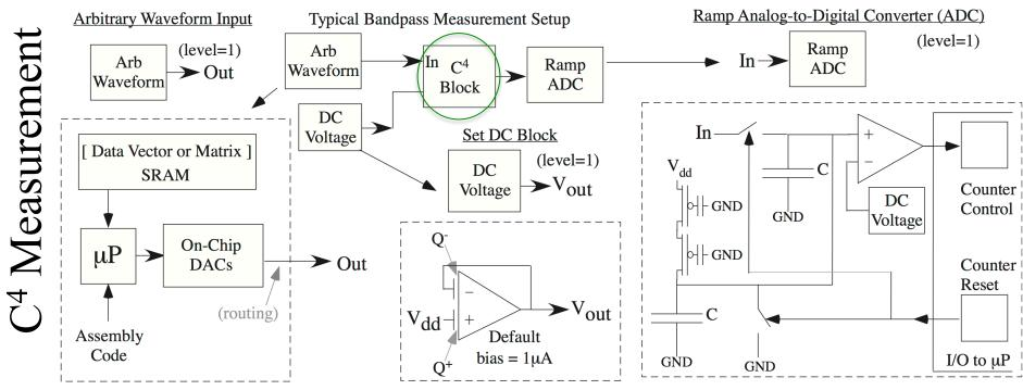
Experimental measurements of C4 Second-Order Section Block, a core signal processing function. and various testing modes.
