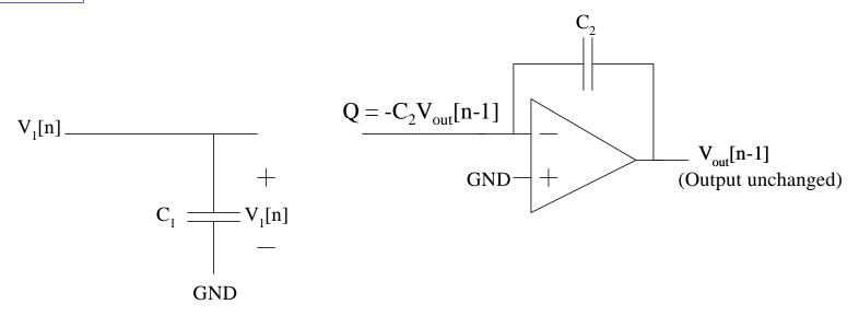
• Charge up the capacitor with voltage V<sub>1</sub>[n]
