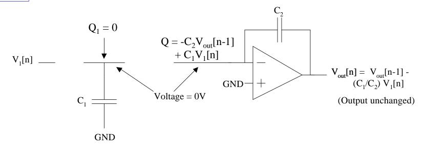
• We disconnect the capacitor from the charge summing node, and return to our initial case
