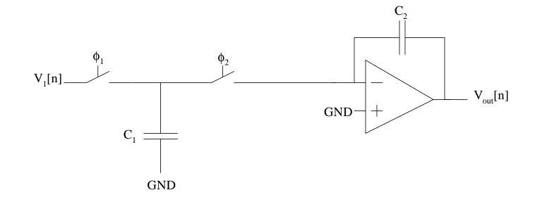
$$V_{out}[n] = V_{out}[n-1] - (C_1/C_2) V_1[n]$$
