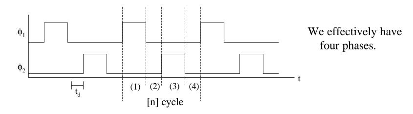
Would want t<sub>d</sub> as small as possible for proper operation
