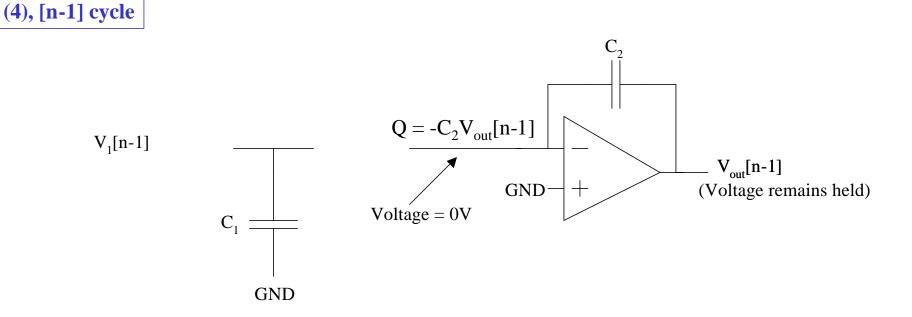
• This case is important to understand our starting point charge is stored on a capacitor ; therefore we need to know the initial state
