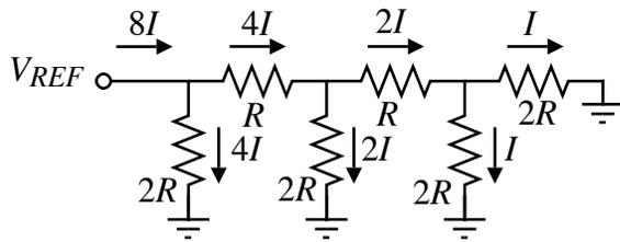
“The resistance seen to the right of any of the vertical  $2R$  resistors is  $2R$ .”
