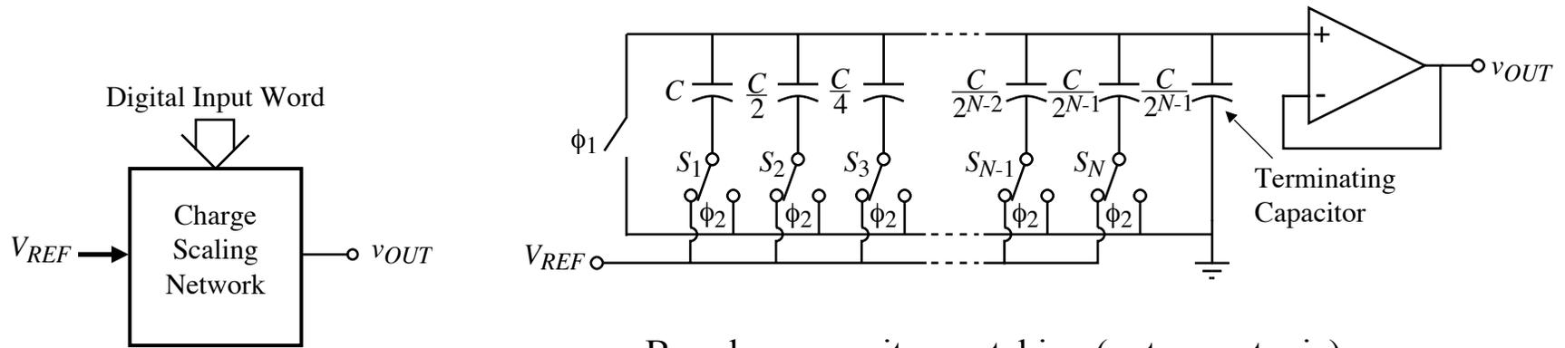
Based on capacitor matching (not monotonic)
