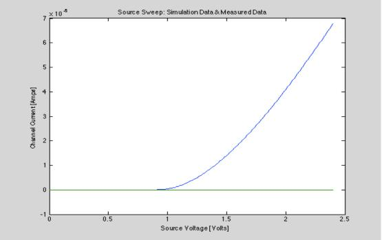
The simulation for the Source sweep did not work, possibly because the biasing voltages were wrong.
