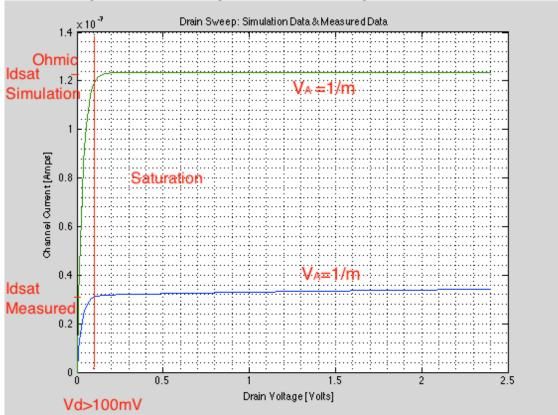
Clearly the simulation data (green) and the measured data (blue) are different. It appears as though the measured data was taken at a lower gate voltage. The measured data is sub-threshold, because the curve saturates at 100 mV.
