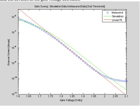
The simulation data gives a good approximation to the measured data, however at higher gate voltages, this approximation is not as good.
