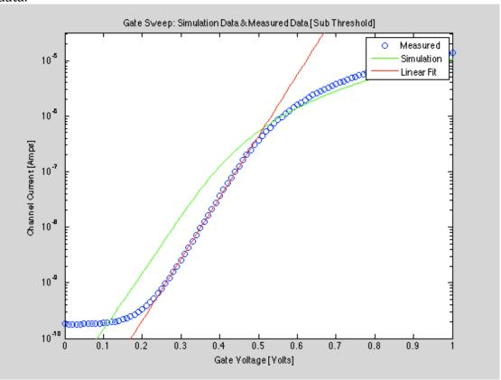
The simulation data deviates from the measured data below the threshold voltage, after the threshold voltage is reached the error of the simulation decreases.
