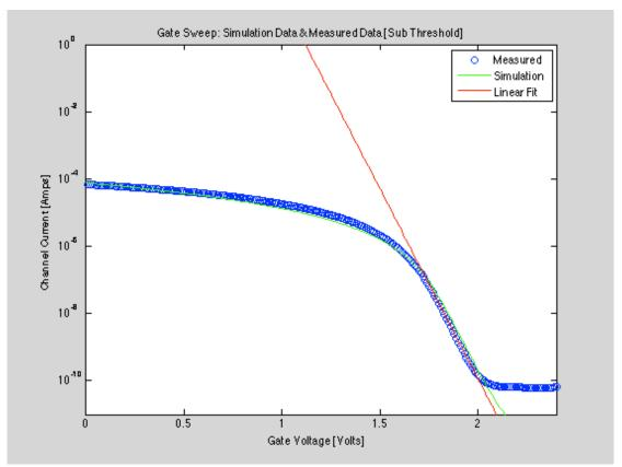
This figure shows how the simulation is a good approximation of the measured data at lower gate voltages.
