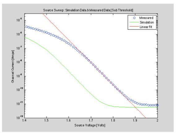
The simulation data deviates from the measured data by approximately 0.1 Volts, however it does follow the same shape.
