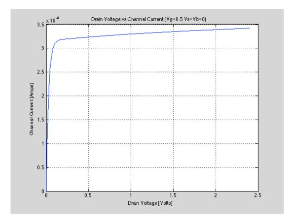
The current at which the curve saturates is below the threshold current, therefore the curve is taken in the sub threshold operation of the MOSFET. It is possible to tell this from the way the curve saturates at greater than 100 mV ( $4U_T$ )
