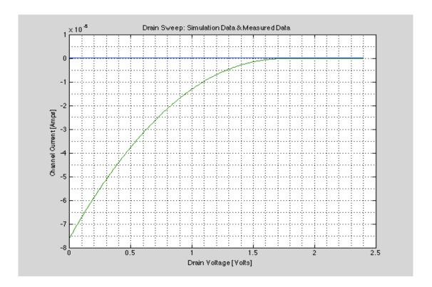
Again the pFET simulation gave results that did not match the measured results. In this case it appears that the simulation pFET was in the above threshold region, while the measured results was identical to the nFET results and was in sub threshold.
