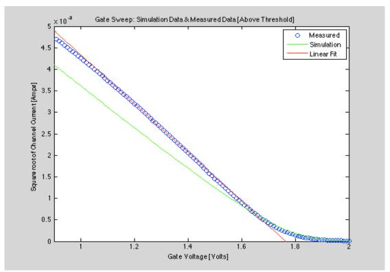
The simulation data gives a reasonably good approximation to the measured data but deviates as the gate voltage decreases.
