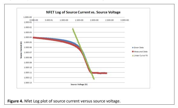
This measured source data was far more accurate than the drain data from figures 2 and 3 in that the curves have similar shapes and remain close together throughout the plot. The linear curve fit also did measure the slope of the linear region adequately. Figure 5 shows the square root plot of source current versus source voltage.
