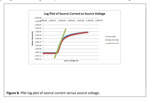
Like the nfet, the source current plots are more accurate than the drain current plots. The plots remain together throughout the entire sweep and the linear curve fit slope is accurate for almost the entire linear region. Figure 9 shows the square root plot of source current versus source voltage.
