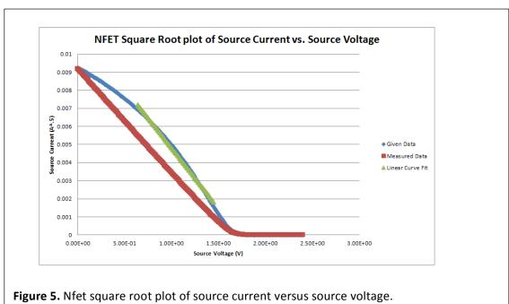
This plot had a similar issue as with the plot in figure 2 in that the given data set is not entirely linear and therefore the linear curve fit and measured data are more linear than the given data. Figure 6 shows the plot of gm versus a logarithmic drain current.
