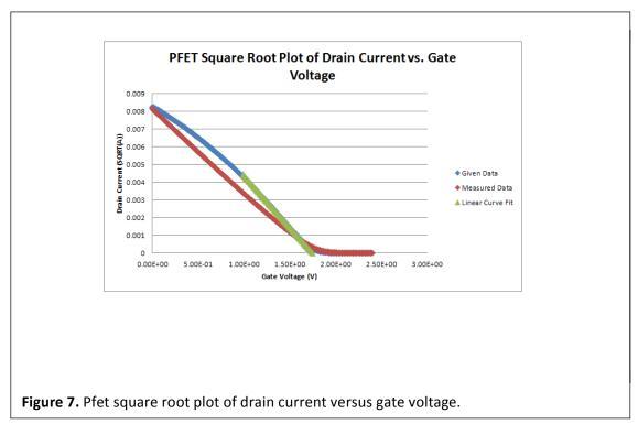
The given data and measured data in figure 7 do line up well in the region past and just before the linear region, but due to the non-linear nature of the given data, the measured data cannot curve to meet the given current measurements. This problem also arises for the linear curve fit trying to fit a non-linear region. Figure 8 shows the logarithmic plot of the source current versus the source voltage.
