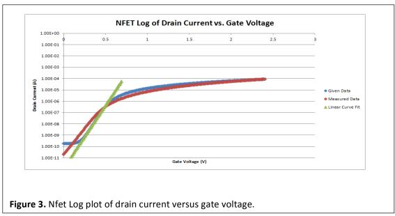
The curve fit for this plot did adequately measure the linear region, but the beginning of the measured data does not appropriately follow the given data as it should. Also please note that for the measurements shown in figures 2 and 3, the value of K was adjusted slightly to  $60 \,\mu\text{A/V}^2$  causing the
