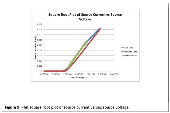
This measured data is close to the given data; however, the K parameter was adjusted to  $60 \,\mu\text{A/V}^2$  and gamma was adjusted to .5 as opposed to being the calculated 1.06. The linear curve fit does give an accurate slope, but only for a section of the linear region and not the entire length. A plot of gm versus a logarithmic current was also taken for the pfet and is shown in figure 10.
