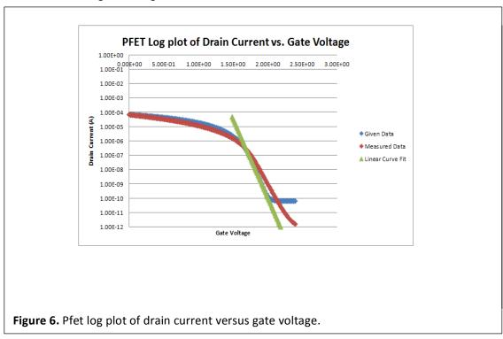
The below threshold region in this plot is adequately simulated by the circuit with the found parameters; however, it begins to deviate at about 1.75 V. The linear region is long enough for the linear curve fit to adequately measure the slope. Figure 7 shows the square root plot of the drain current versus the gate voltage.
