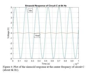
By changing the resistance we could manipulate the Q-factor without changing the time constant. A resistance less than 61 ohms would yield a Q-factor of less than  $\frac{1}{2}$  and give us complex roots. We replaced the 1k ohm resistor in circuit C (Figure 3) with a trimpot so we can adjust the resistance in the circuit and see changing responses.
