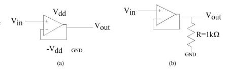
Figure 1: The schematic of the first two circuits used in this lab. Both are op-amp buffer circuits in which Vout is approximately equal to Vin.
