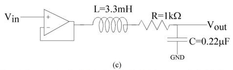
Figure 3: The schematic of the third circuit used in this lab. It is an op-amp buffer linked into a second order low pass filter LRC circuit.
