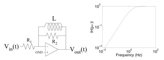
Question 8: (True/False) The circuit has the resulting frequency response shown for  $R_1 = R_2$ .
