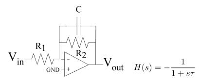
Question 3: (True/False) The circuit has the resulting H(s) transfer function for  $R_1 = R_2$ .
