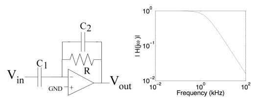
Question 6: (True/False) The circuit has the resulting frequency response shown for  $C_1 = C_2$ .
