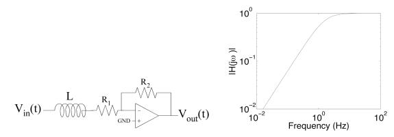
Question 7: (True/False) The circuit has the resulting frequency response shown for  $R_1 = R_2$ .
