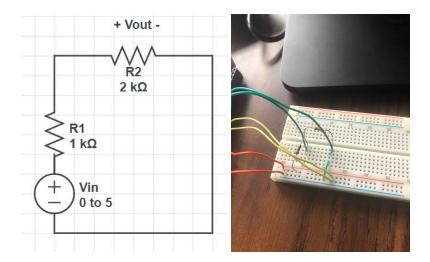
Figure 1: Voltage divider diagram and circuit
